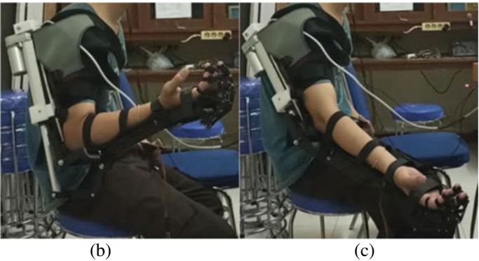
Fig. 5 a Elbow exoskeleton design using linear actuator, b linear actuator push the arm (flexion position), and c linear actuator pull the arm (extension position)
