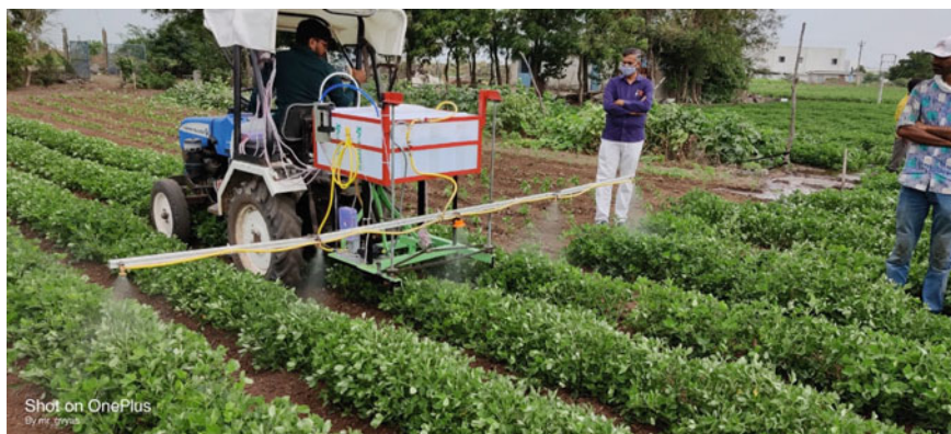
Fig. 11 Field test of pesticide filling and spraying attachment
