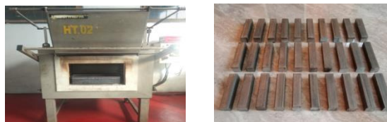
Gambar 2. Tungku Pemanas Nabertherm Made In Germany dan Material Baja ST 60
