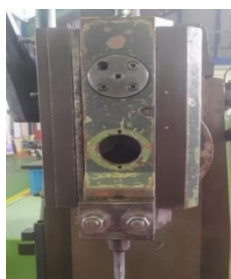
(a) Slotting Attachment kondisi baik
